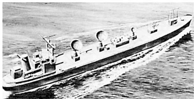
Figure 2—Drawing of completed Apollo program ship providing insertion/injection coverage.
