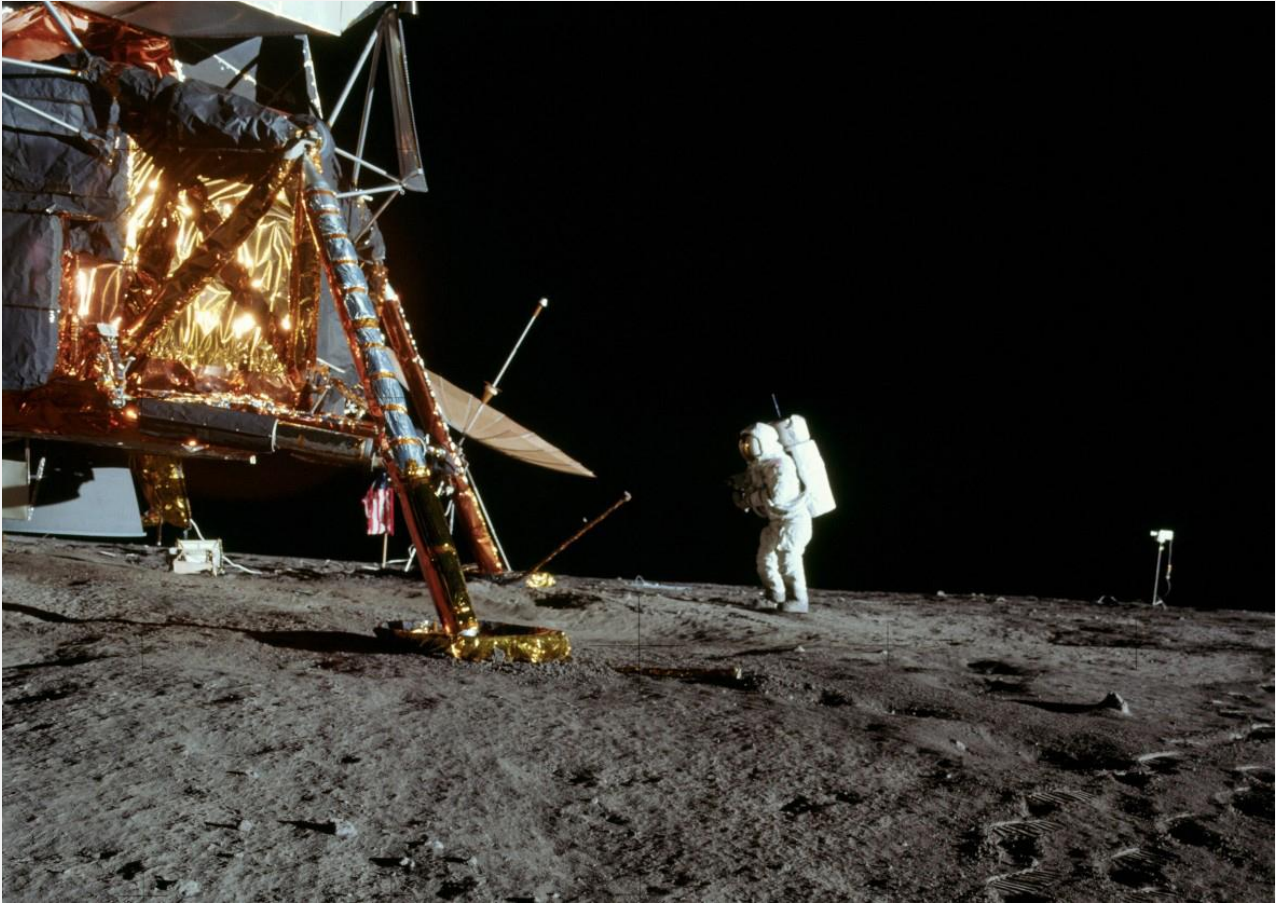
Alan Bean with the TV camera behind him. The erectable S-band antenna is pointing straight at Earth. Image: NASA - AS12-46-6779
