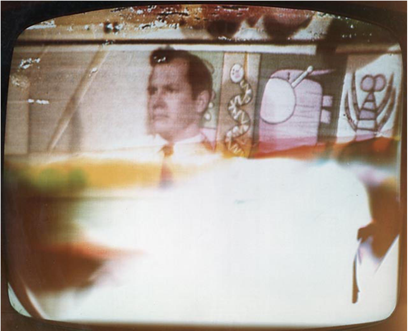
The camera target, although damaged, still worked. Photo courtesy of Stan Lebar, Westinghouse Lunar TV Camera Program Manager.
