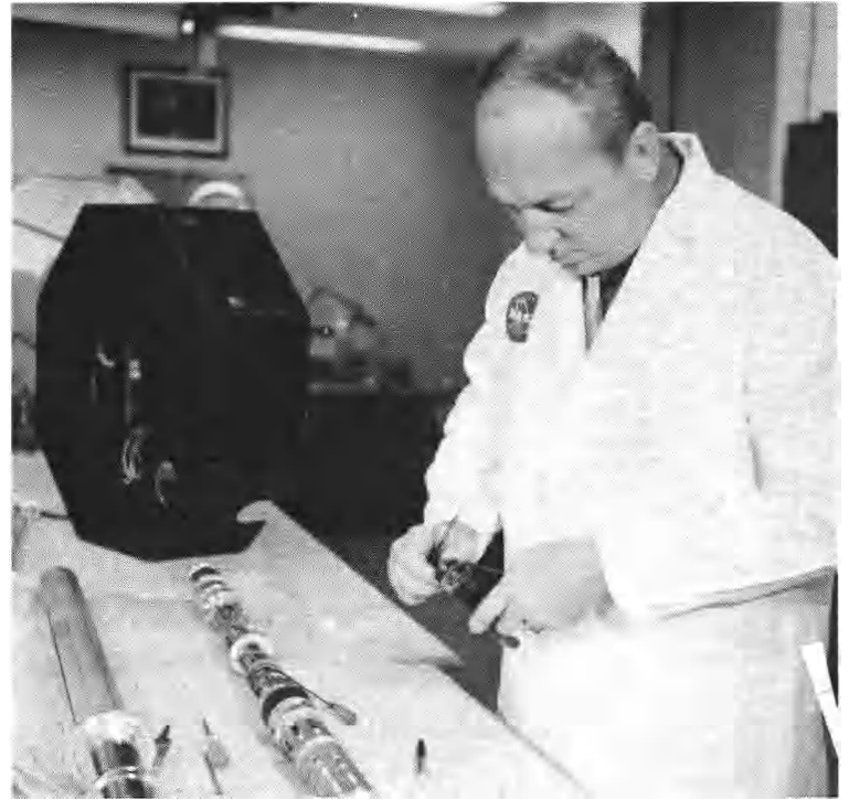
Ray Berkley is assembling the Rubidium vapor magnetometer.
