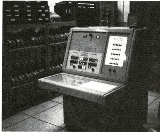
The Launch Operations Manager's Console is continuously monitored to detect any indication of an emergency situation. The photo below is a blowup of the console panel.
