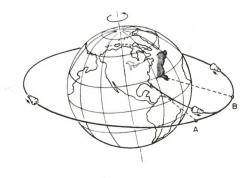
In this drawing, one orbit is from point A, around the earth, and back to point A. Since the longitude of Cape Kennedy has rotated about 23 degrees to the East (point B), one revolution has not been considered completed until the spacecraft has traveled this additional "Distance" and is again over the longitude of Cape Kennedy.
