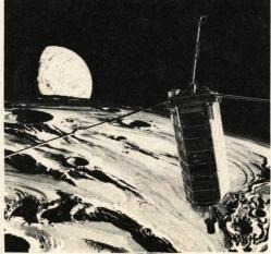
An artist's concept of the P&FS satellite, which will carry particle detectors and magnetometers to obtain information about the interaction of the earth's magnetic field with the moon. The satellite will be carried in a service module compartment on the Apollo 15 mission.
