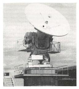
This CAPRI radar at TAN gives precession tracking of space vehicles in both range and angle. TAN tracking of the Apollo spacecraft is vital during earth orbital periods.
