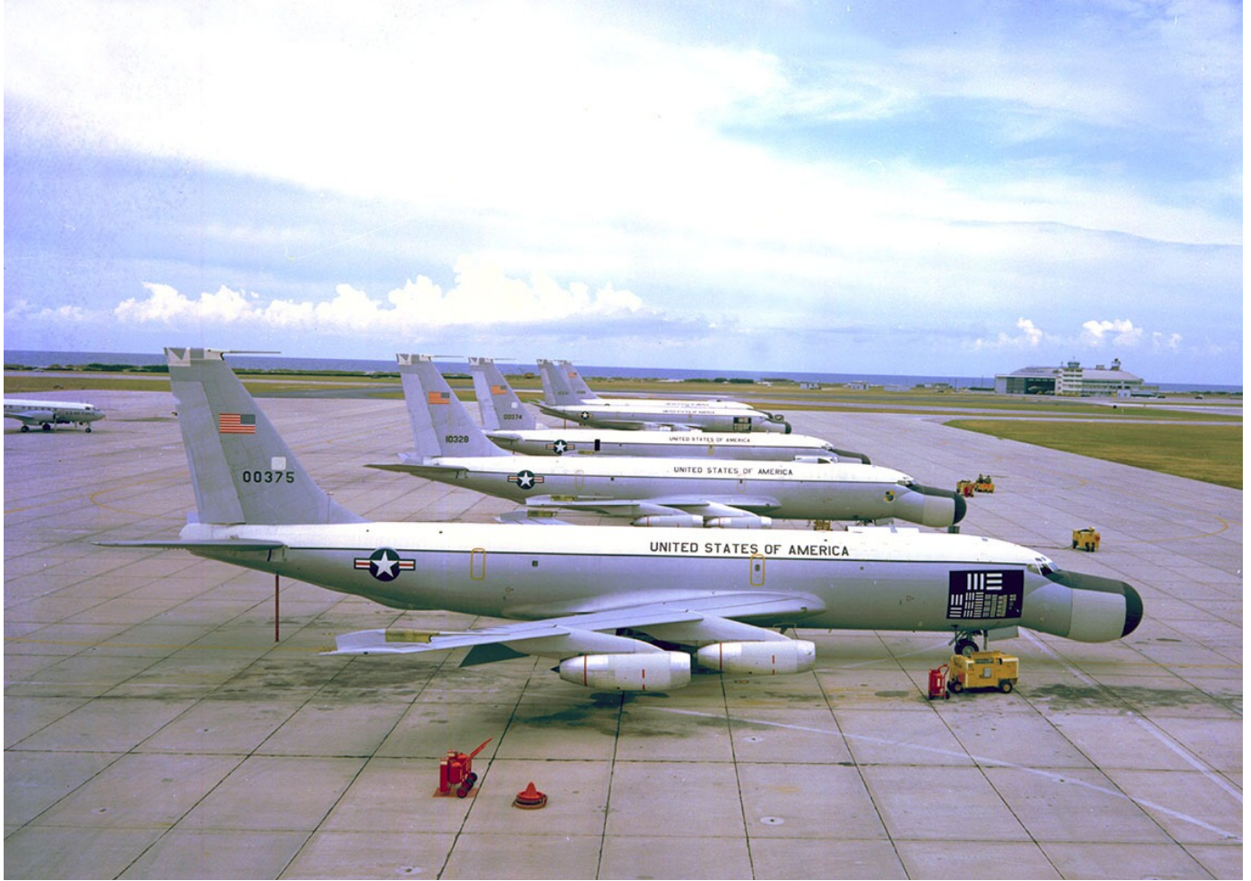
Figure 4: Five ARIA on the tarmac at Patrick AFB facing south. Hangar 800 and Atlantic Ocean in background ( photo by Bob Burns). Note ARIA TN 375, ARIA #1 for Apollo 17 TLI, has the special paint scheme for calibrating the ALOTS while in flight. ARIA TN 328, ARIA #2 for Apollo 17 TLI and reentry is ALOTs capable with special radome on top of fuselage located at FS 600. The ALOTS radome was successfully used for realtime satellite retransmission of telemetry data
