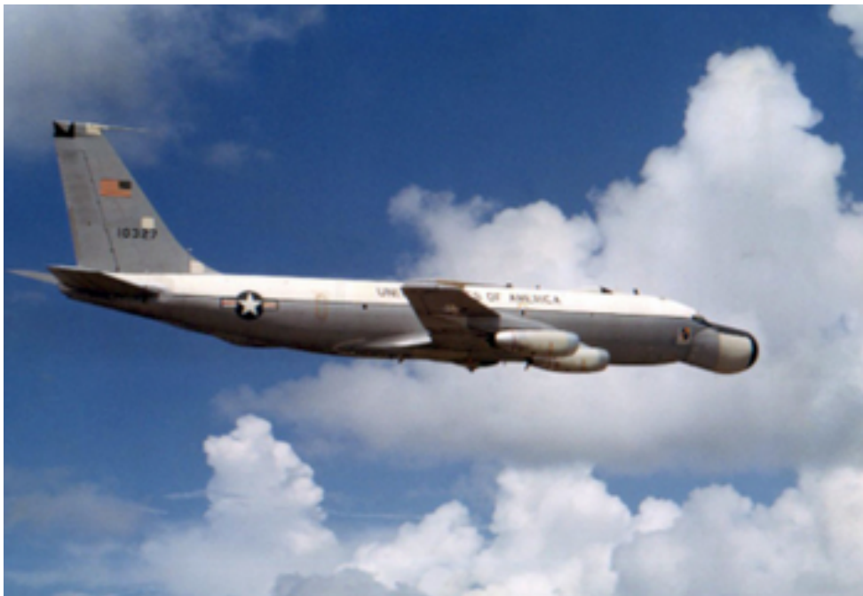
Figure 2: ARIA 61-0327 (Boeing C/N 18234) in flight off Patrick Air Force Base (note: “A”model engines, USA flag carrying diplomatic paint scheme, HF wing tip probes, ALOTS radome)
