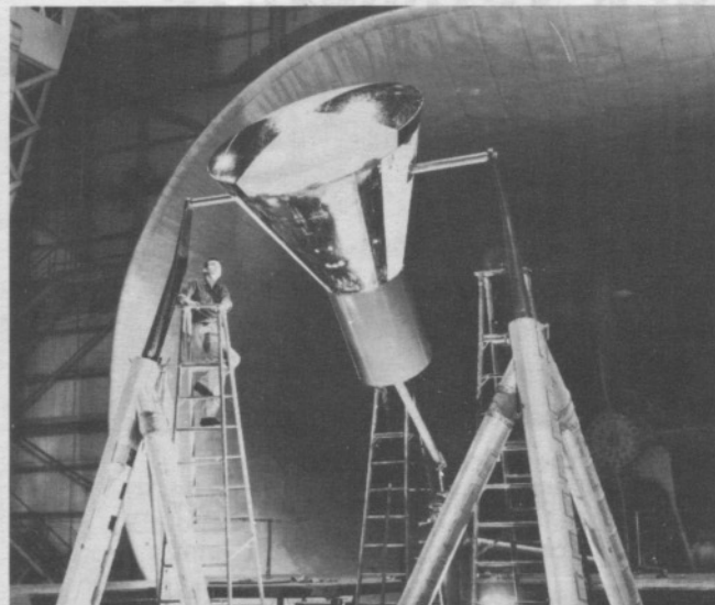
To determine the space capsule's lift, drag and other characteristics in flight, tests were made in a wind tunnel which simulated an airspeed of 28,000 kilometers per hour.
