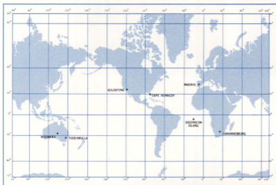
DSIF stations circle the globe at intervals of 120 degrees in longitude to maintain continuous coverage of the spacecraft.
