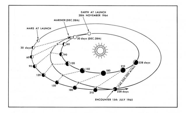
FIGURE 5. MARINER TRAJECTORY TO MARS
