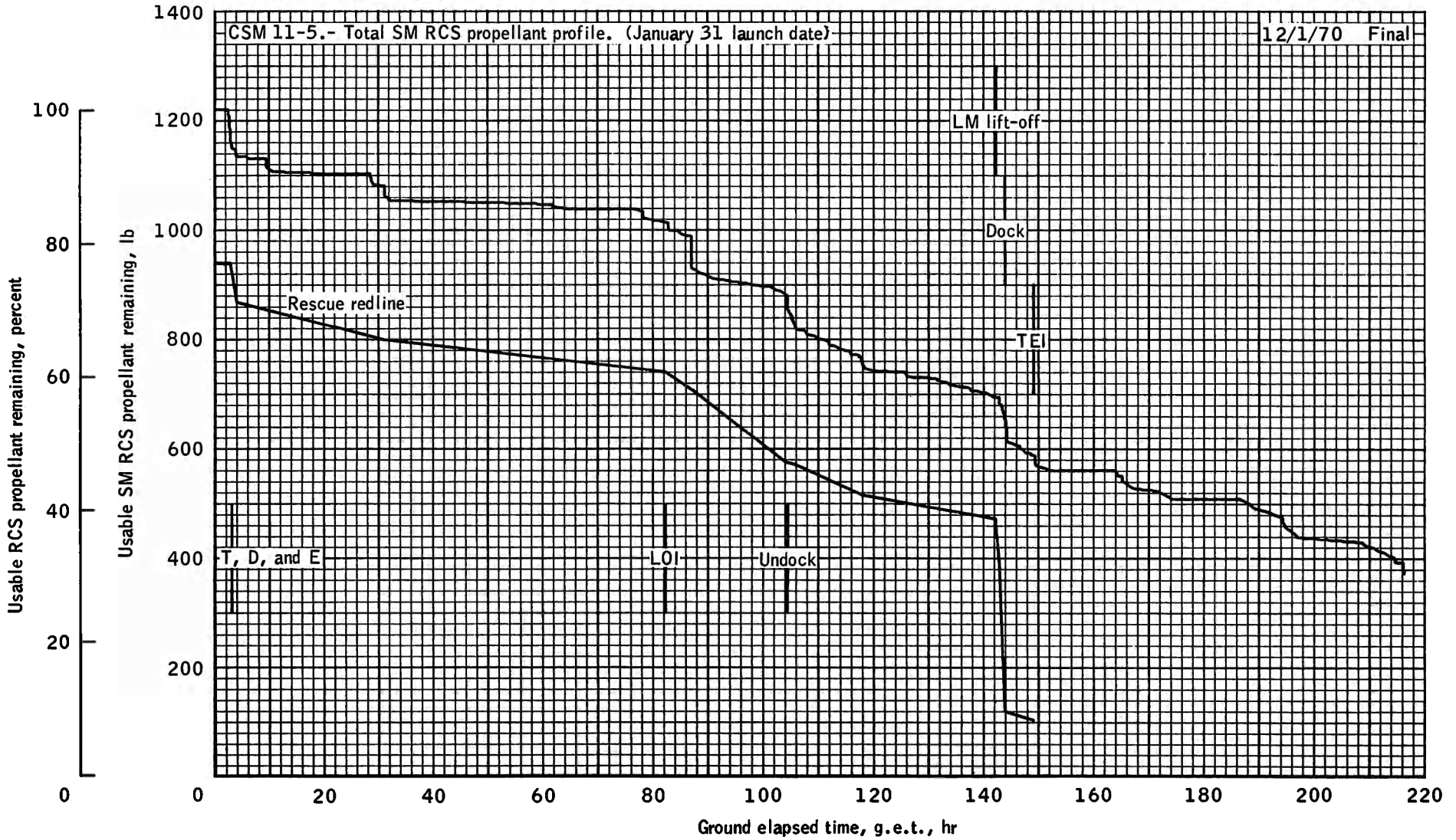
Figure 4-10.- Total SM RCS propellant usage profile.
