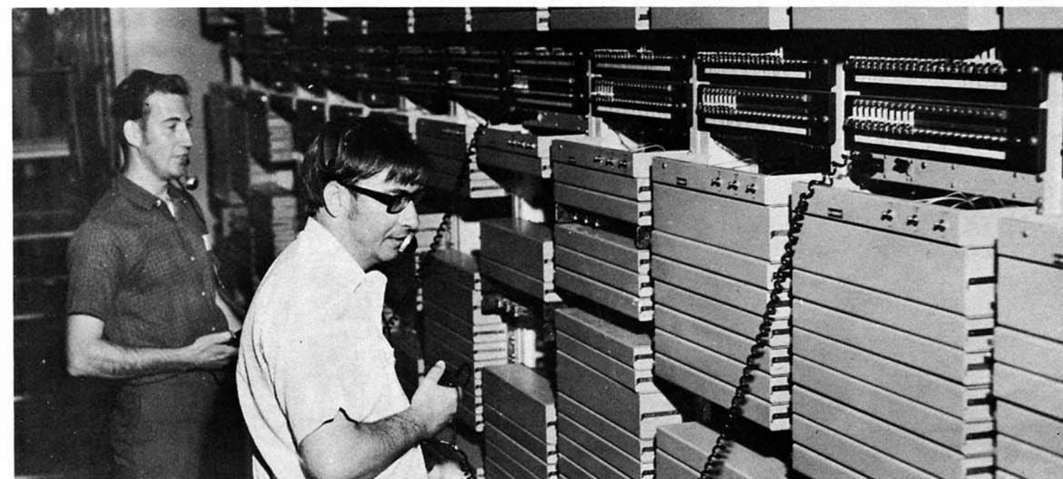
'VERIFY, PLEASE' — Technical Writers Ray Buchheister (left) and Bob Runion check the relays in the Interphone subsystem onboard NASA's Vanguard tracking ship.
