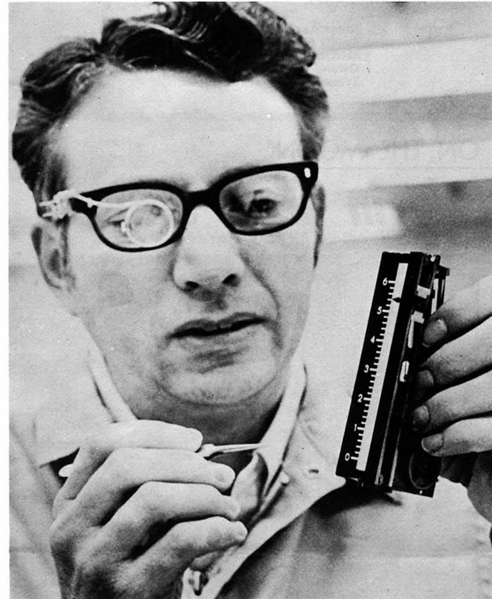
APOLLO PLUMB BOB — A thrust-to-weight-ratio indicator was used by Apollo 11 astronauts to monitor the thrust of ascent and descent engines during the lunar landing phase of the epic moon flight. The pointer moves along a fixed vertical scale that is calibrated from zero to 6.5 lunar-gravity-units.
